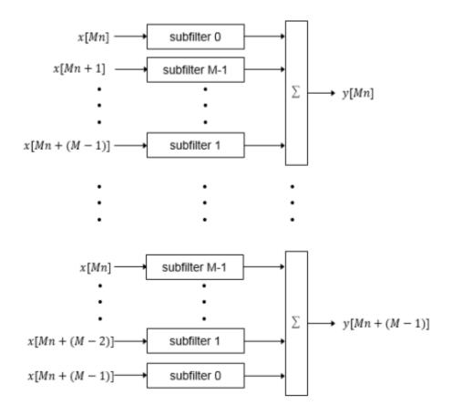
Each of the subfilters includes every *M*th coefficient. The subfilter results are added so that each output sample is the sum of each of the coefficients multiplied with one input sample.
