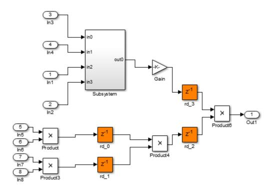
The subsystem now contains pipeline registers:
