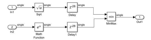
When generating HDL code, the generated model shows how HDL Coder implemented the floating-point operators.
