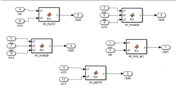
For example, the ml\_mul\_acc MATLAB Function block shows how to write a multiply-accumulate operation in MATLAB. hdlfimath on page 20-36 applies fixed-point math settings for HDL code generation.
