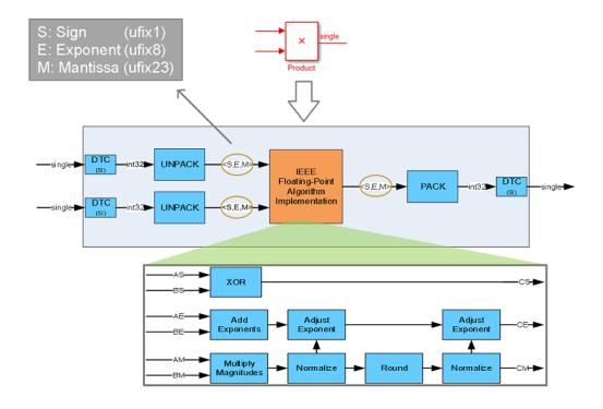
The Unpack and Pack blocks convert the single-precision types to the sign, exponent, and mantissa. In the figure, S, E, and M represent the sign, exponent, and mantissa respectively. This interpretation is based on the IEEE-754 standard of floating-point arithmetic.
