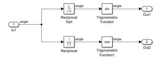
After HDL code generation, the generated model shows the native floating-point operators corresponding to the blocks in your Simulink model.
