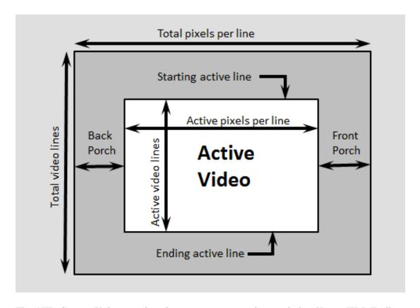
The AXI4-Stream Video interface does not require a video porch, but Vision HDL Toolbox algorithms require a porch for processing video streams. If the incoming pixel stream does not have a sufficient porch, HDL Coder inserts the required amount of porch to the pixel stream. By using the AXI4-Lite registers in the generated IP core, you can customize these porch parameters for each video frame:
