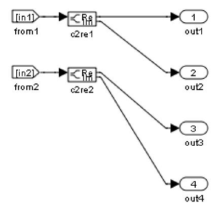
The model maintains the separation of real and imaginary components throughout the cosimulation path. The Compare subsystem performs separate comparisons and separate scope displays for the real and imaginary signal components.
