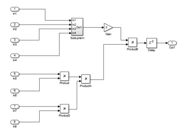
The following diagram shows the generated model after distributed pipelining redistributes the delay to reduce the critical path.
