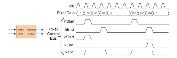
The **Pixel Data** signal is the primary video signal that is transferred across the AXI4-Stream Video interface. When the **Pixel Data** signal is valid, the **valid** signal is asserted.
