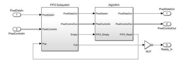
The **FIFO Subsystem** block uses HDL FIFO blocks for the **Pixel Data** and for the **Pixel Control Bus** signals.
