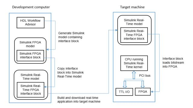
This example uses the Speedgoat IO331. You can use any FPGA I/O module supported by Simulink Real-Time and HDL Coder that meets the speed, size, and pinout requirements of the model.
