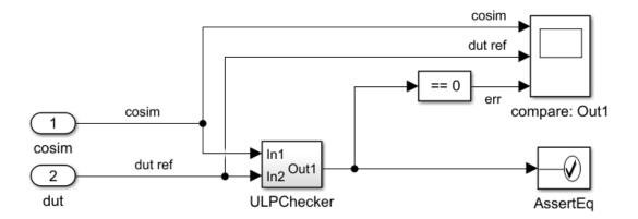
The ULPChecker has a MATLAB Function block that shows how HDL Coder accounts for the ULP error when checking for numerical accuracy.
