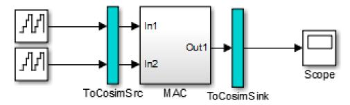
The two subsystems labelled ToCosimSrc and ToCosimSink do not change the performance of the simulation path. Their purpose is to capture stimulus and response signals of the DUT and route them to and from the HDL cosimulation block (see "Signal Routing Between Simulation and Cosimulation Paths" on page 18-49).
