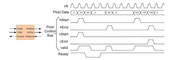
When you map the DUT ports to an AXI4-Stream Video interface, you can optionally model the backpressure signal, **Ready**, and map it to the AXI4-Stream Video interface.
