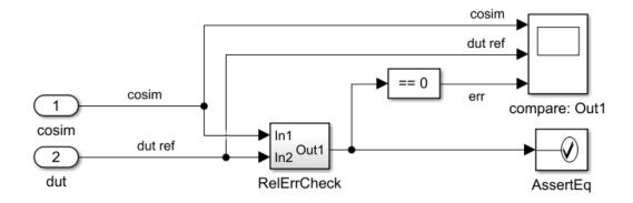
RelerrCheck has a MATLAB Function block that shows how HDL Coder accounts for the relative error when checking for numerical accuracy.
