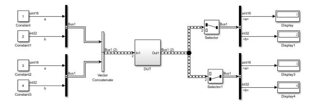
The array of buses combines two nonvirtual bus elements, each having scalars a and b of types uint16 and int32 respectively.
