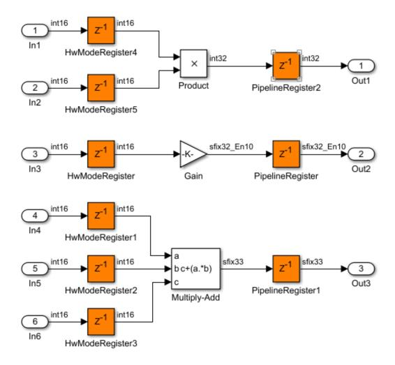
The pattern and number of pipeline registers that HDL Coder inserts can vary depending on the target device, target frequency, and the multiplier word lengths.
