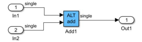
**2** Double-click the **ALT add** block. The length of the delay block is the latency of the floating-point target IP.
