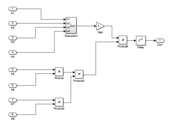
The following diagram shows the model after applying hierarchical distributed pipelining:
