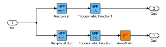
To get the latency information of the floating-point operator, double-click that **NFP** block. For example, if you double-click the **NFP sqrt** block, you can get the latency of the floating-point reciprocal square-root implementation. Here, the latency is 17.
