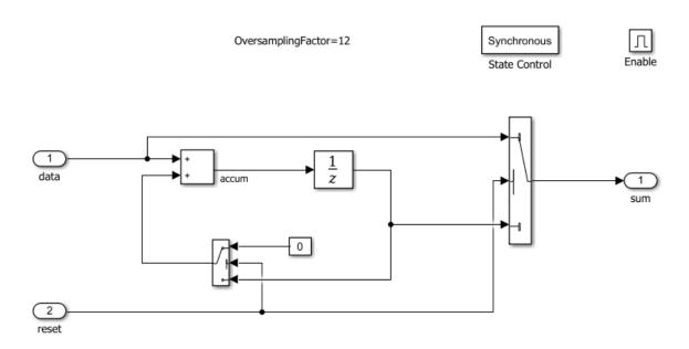
The Add block has a maximum latency of 12. When generating code, HDL Coder<sup>™</sup> cannot allocate 12 delays for the block, because it cannot add matching delays to other paths.
