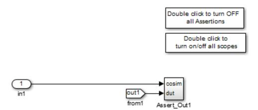
For each output of the DUT, HDL Coder generates an assertion checking subsystem (Assert\_OutN). The subsystem computes the difference (err) between the original DUT output (dut ref) and the corresponding cosimulation output (cosim). The subsystem routes the comparison result to an Assertion block. If the comparison result is not zero, the Assertion block reports the discrepancy.
