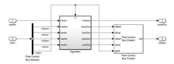
You can directly connect the **valid** signal from the **Pixel Control Bus** to the Enable port. If you do not have the Vision HDL Toolbox software, replace the Pixel Control Bus Selector and Pixel Control Bus Creator blocks with the Bus Selector and Bus Creator blocks respectively.
