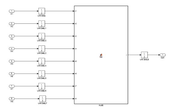
The following shows a chain of multiplications as coded in the  ${\tt mult8}$  MATLAB Function block:
