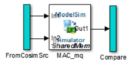
The FromCosimSrc subsystem receives the same input signals that drive the DUT. In the gm\_hdl\_cosim\_demo1\_mq0 model, the subsystem simply passes the inputs on to the HDL Cosimulation block. Signals of some other data types require further processing at this stage (see "Signal Routing Between Simulation and Cosimulation Paths" on page 18-49).
