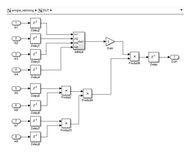
The subsys block in DUT contains a copy of the three Product blocks in the lower half of the diagram.
