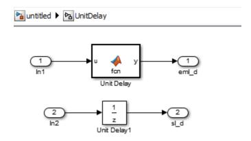
The MATLAB code in the MATLAB Function block uses a persistent variable to model the register.
