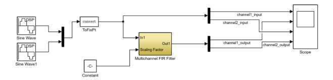
The model includes a two-channel sinusoidal signal source feeding a filter subsystem targeted for  $\rm HDL$  code generation.
