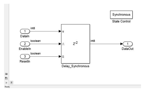
The SynchronousStateControl and ClassicStateControl subsystems use a Delay block with an external reset and an enable port in Synchronous and Classic modes respectively.
