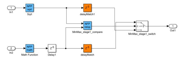
The **NFP Sqrt** block has a maximum latency of **28**. This latency is equal to the **Delay length** of the Delay block at the output of your Simulink model. HDL Coder absorbs the Delay inside the **NFP Sqrt** block.
