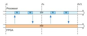
If you use vector data signals at the DUT interface, the IP core report displays this section that shows how the code generator synchronizes vector data across the AXI4 interface.
